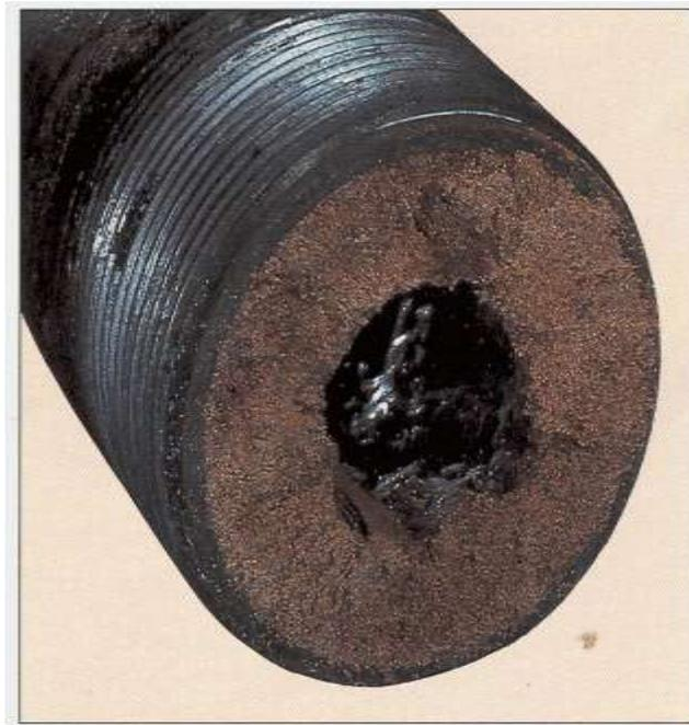
*Figure 1. APWD causing complications in work of wells.*
