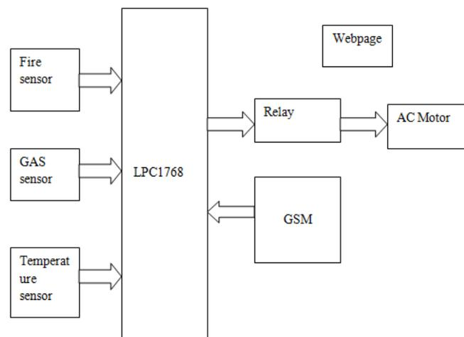
**Fig 3: Block diagram of weather monitoring**
