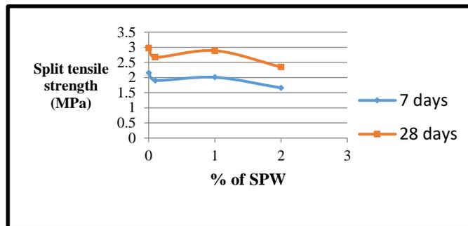
Figure 3. Split tensile strength vs % of SPW
