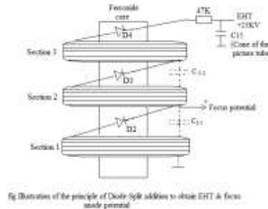
Fig Illustration of the principle of Diode Split addition to obtain EHT & focus anode potential
