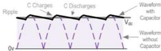
Fig17. Rectifier Output Waveform
