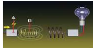
*Fig2. Induction Principle*
