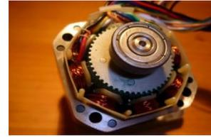
Figure 7. Stepper Motor
