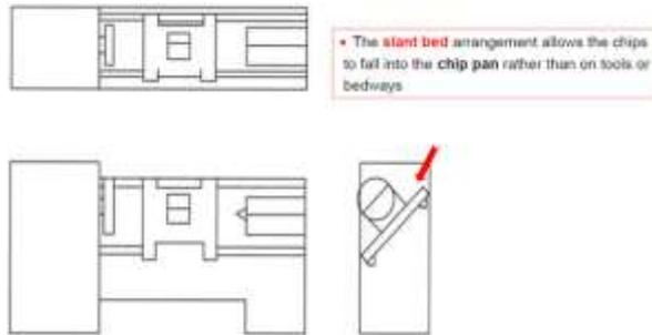
Fig. 2 Slant Bed arrangement for NC or CNC lathe
