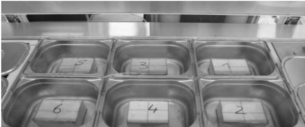
Figure 2: Determination of the capillary suction of de-icing solution and freeze thaw test
