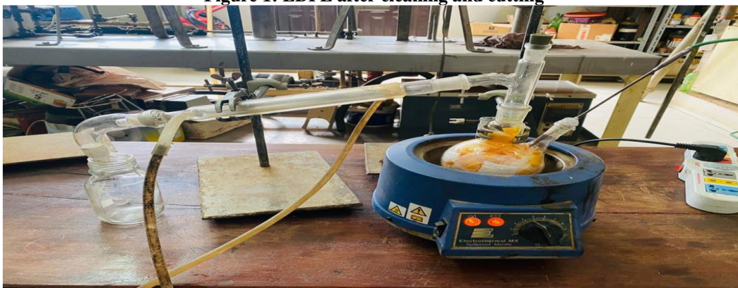
Figure 2: Pyrolysis process for conversion of waste plastic into fuel
