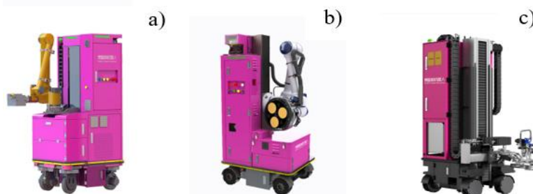
Figure 5: Caulking, sanding, and painting robots[13]
